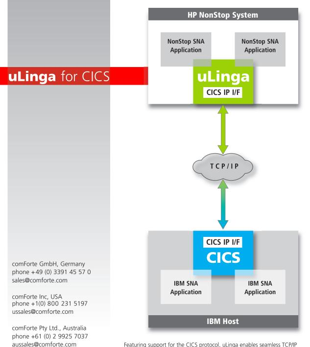
Featuring support for the CICS protocol, uLinga enables seamless TCP/IP communications between HP NonStop platforms, and IBM mainframes.
